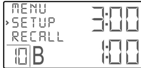
Only 3 lines of each menu will be on the screen at any one time and they are located on the top left part of the LCD screen. The > located at the center line indicates what will be activated when you push the **SET** button. The remaining will be off-screen and you will use the **V** or **Λ** buttons to scroll the menu to access them.
